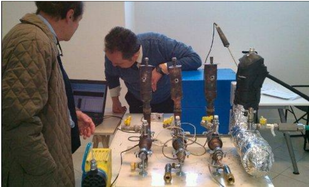
Figure 1 showing Andrea Rossi (left) and Giuseppe Levi (right). Shown are the water pump in yellow, three bare Rossi devices (ECATS) and one heat-insulated Rossi device (ECAT) which was used for the experiment. In the middle of the horizontal section is seen the container ca 50 cm 3 in volume with the hydrogen gas-fill pipe on its top. The electric heater is connected at the end of the horizontal section. The chimney is used for the steam accumulation. (Photo: Sven Kullander).
