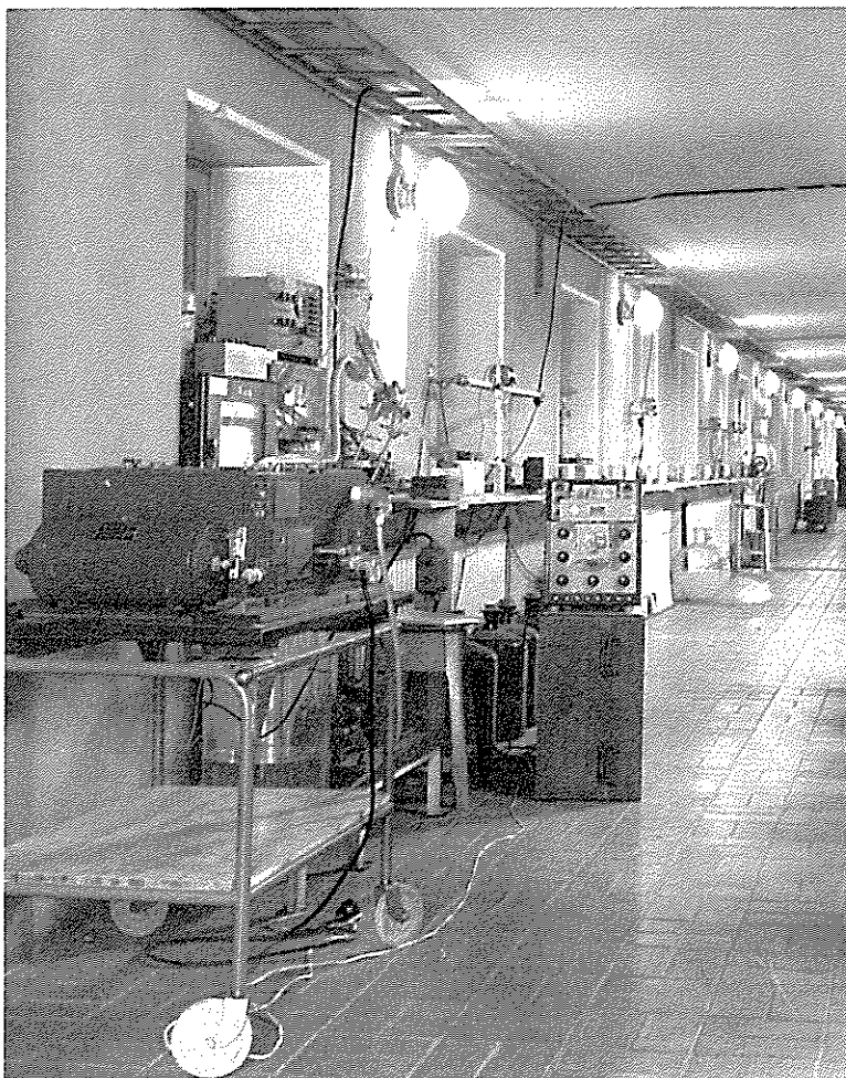
Fig. 4.2. Photograph of the complete experimental equipment including also measuring components used for pressure drop measurements reported in Part 5 of the paper.
