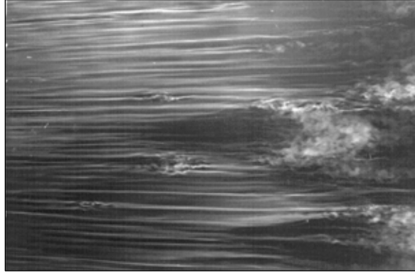
FIGURE 2.6. Smoke visualisation of streaks in the boundary-layer induced by free-stream turbulence. Flow is from right to left. From Matsubara et al. (1998)
