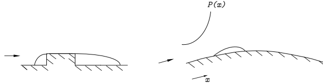
FIGURE 2.1. Two classes of separation: geometry-induced and adverse pressure gradient-induced separation
