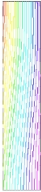
FIGURE 2.2 The iso-contours of the electric potential in an enclosed electrochemical cell. Calculations performed with CFX of a laminar case. -7.0 \cdot 10^{-2} \text{ V} \leq \Phi \leq +7.0 \cdot 10^{-2} \text{ V} .
