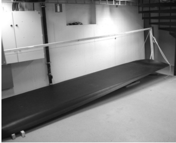
Figure 20. The inclined ground plane. The inclination is adjustable by changing the height at one end. The walker is attached to the safety wire via a slack rope and a pulley.
