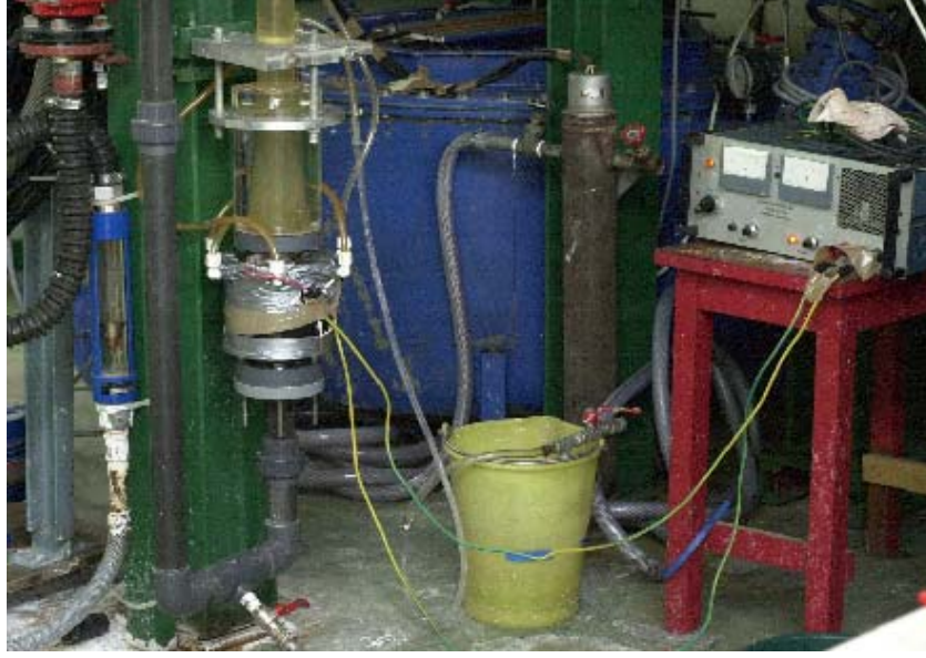
FIGURE 4.3. The Electrochemical Bubble Appliance, EBBA, mounted in the lower part of the pipe. The flow-meter is located to the left in the picture, and the rectifier is to the right.
