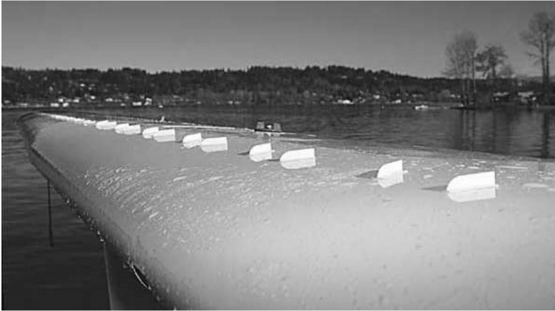
Figure 3.2: Vortex generators in aeroplane use. Reproduced from [61].
