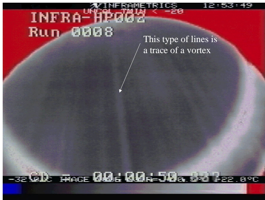
Figure 87. Infrared image: DLR TOP nozzle, vortex origin shortly after nozzle throat, experiment by Stark et al R 123 . (Courtesy of DLR and ASTRIUM)
