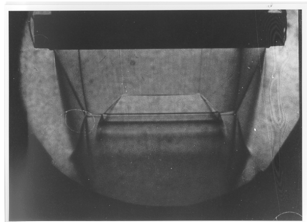
Figure 20 : Schlieren picture at exit for full-flowing conditions, dual-bell nozzle.
