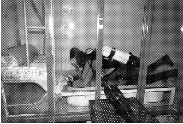
Figure 3.2. Closing the momentum balance. Diver in tank during slot height measurements.
