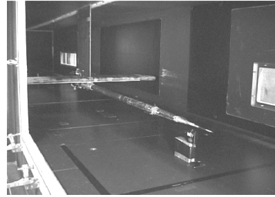
FIGURE 4. Traversing system and probe. The laser distance meter used to check the system vibrations is visible under the probe.
