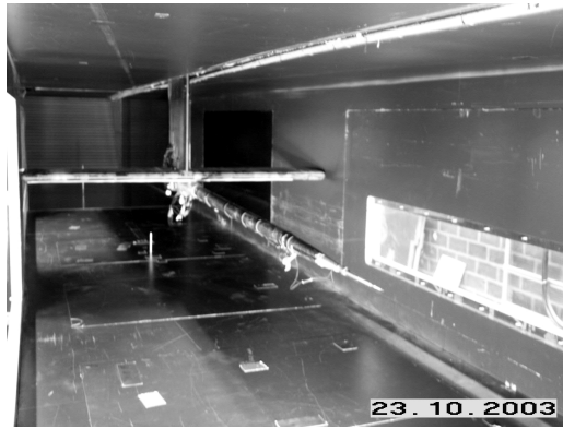
FIGURE 4.2. Test section with traversing system as seen from upstream.
