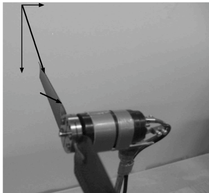
FIGURE 2.1. The angle between the plane of the rotor and the local wind direction is decreasing as moving towards the tip. The stall starts from the root.
