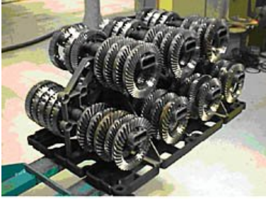
(a) Automotive ring gears vacuum carburized at 1230 K in 114 min cycle with 15 bar nitrogen quench
