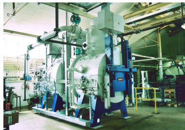
FIGURE 2.2. Two-chamber VAK furnace.
