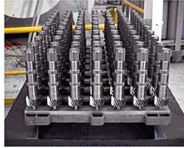
(b) Helical shafts carburized at 1230 K in 114 min cycle with 8 bar nitrogen quench
