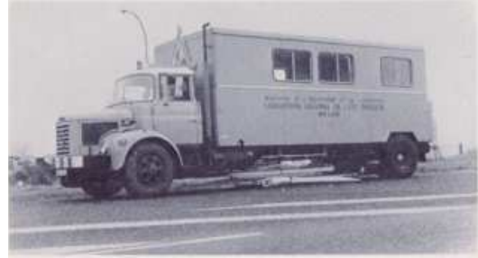
(a) The third Lacroix (1964), built on a Berliet GLM 10 M2 truck. (Reproduced from [135].) (b) The Lacroix Deflectograph 04. (Reproduced from [33].)
