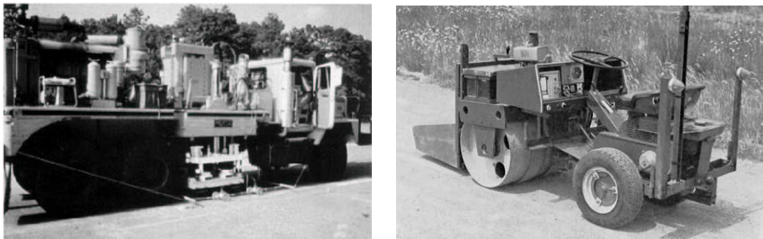
(a) The Rolling Dynamic Deflectometer. (Reproduced from [35].) (b) The Collograph. (Reproduced from [43].)
