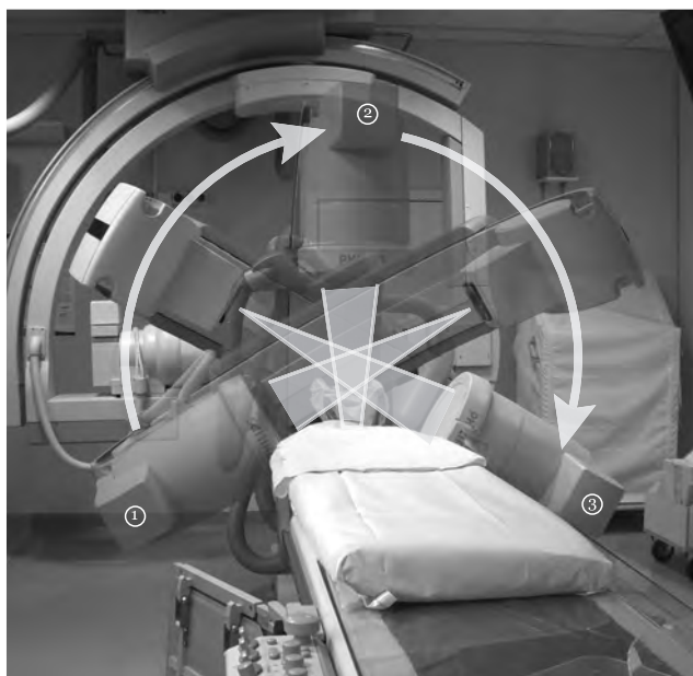
FIGURE 4.5. Motion of the C-arm during a rotational scan. The initial (1) and terminal (3) positions are shown together with one intermediary (2) position. A conical beam is emitted from the source and penetrates the object to be studied.
