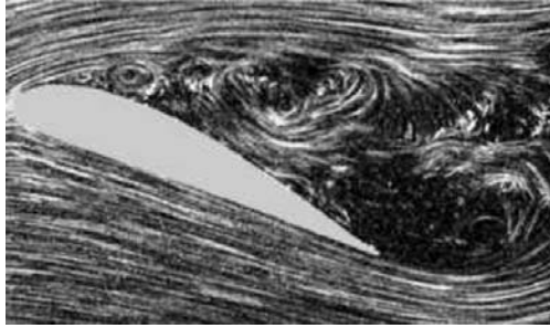
FIGURE 1.2. Flow separation on a wing at high angle of attack.
