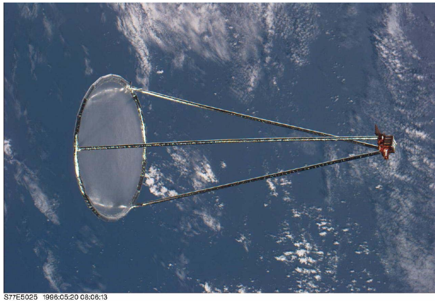
FIGURE 2.12. The Inflatable Antenna Experiment (Courtesy of L'Garde).
