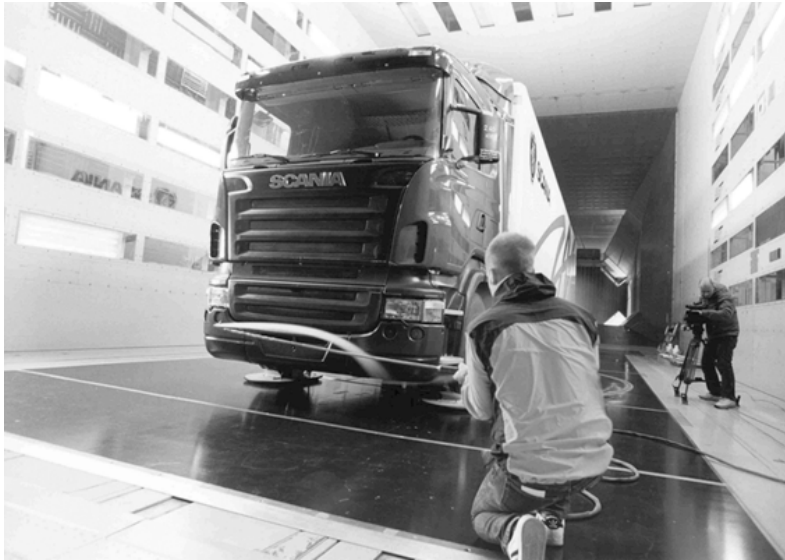
FIGURE 1.1. The author performing a smoke visualisation on a Scania truck in the German-Dutch LLF wind tunnel in 2001. The largest test section, with a cross sectional area of 9.5 \text{ m} \times 9.5 \text{ m} is used for this test.
