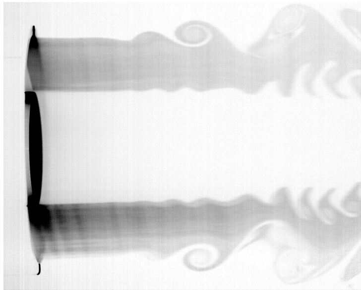
FIGURE 4. Smoke flow visualisation at U_o = 4 m/s and r_u = 1 for the sharp wall.
