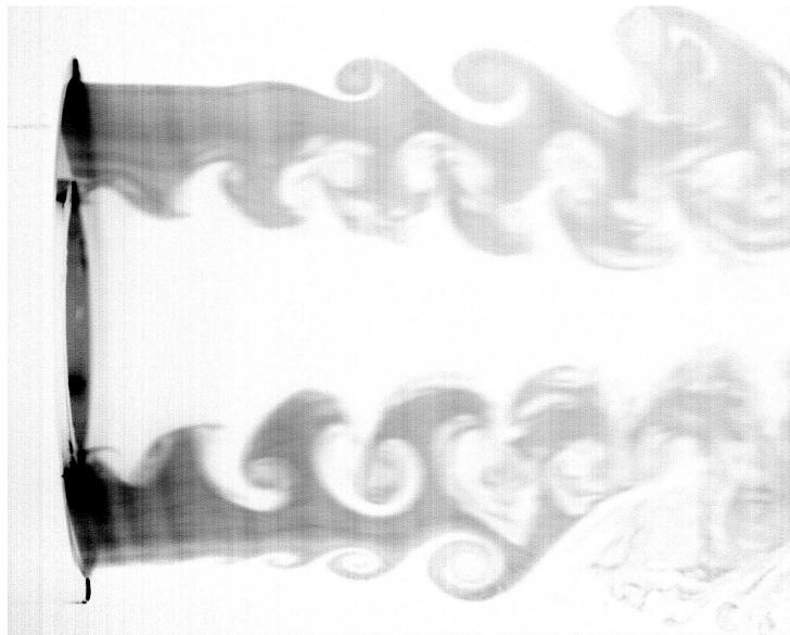
FIGURE 6. Smoke flow visualisation at U_o = 4 m/s and r_u = 1 for the thick wall.
