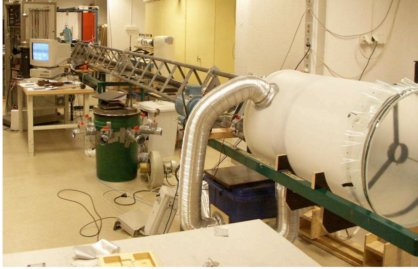
FIGURE 4.3. Experimental setup showing the pipe mounted within the triangular shaped framework and fed into the stagnation chamber covered by an elastic membrane.
