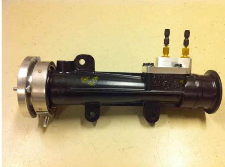
FIGURE 4.6. Photo of the venturi flowmeter. The flow direction is from the right to the left.
