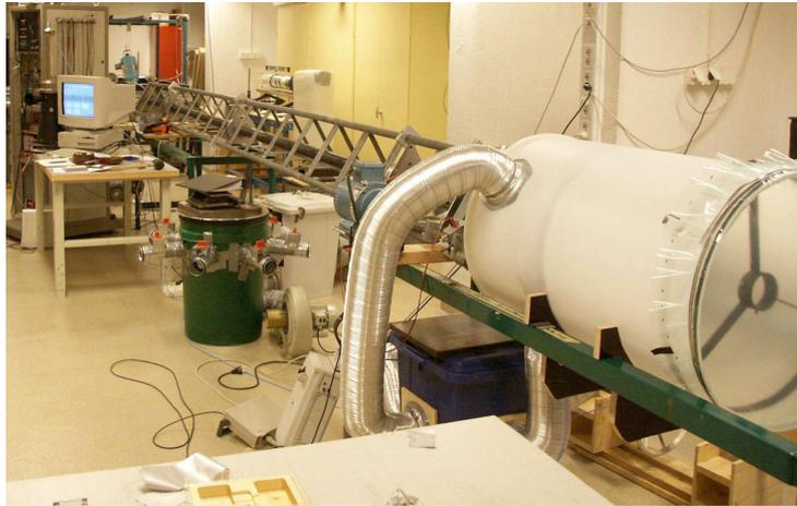
FIGURE 3.1. Close-up of the set up showing the rotating pipe mounted within a triangular shaped framework and connected to the stagnation chamber covered by an elastic membrane in order to further reduce pressure fluctuations.
