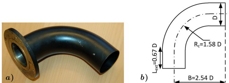
FIGURE 2. *a)* Pipe bend that was mounted at the exit of the  $100 D$  long straight pipe. *b)* Dimensional details of the pipe bend.
