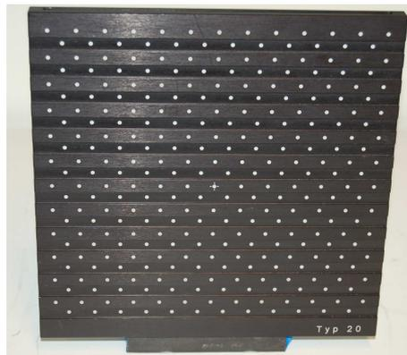
FIGURE 3.18. Two-level calibration plate provided by LaVision GmbH. Levels are separated by 2 mm, dots are equally spaced within 15 mm from each other.
