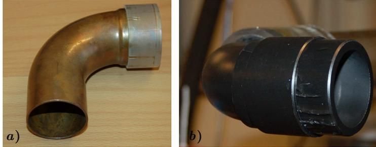
FIGURE 3.7. The two bend pipes used for the measurements performed in the CICERO laboratory. *a)* Bend I *b)* Bend II with the  $1 D$  extension mounted on it.
