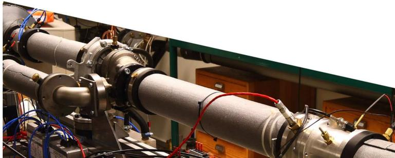
FIGURE 2. Set up for the instantaneous pressure and mass flow rate measurements across the turbocharger (Garrett).
