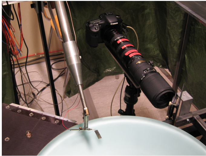
FIGURE 3.5. The typical hot-wire calibration set-up. The hot-wire sensitive area with a precision gauge block put next to the hot-wire probe is captured by a digital camera with a micro lens through the mirror put in the optical path.
