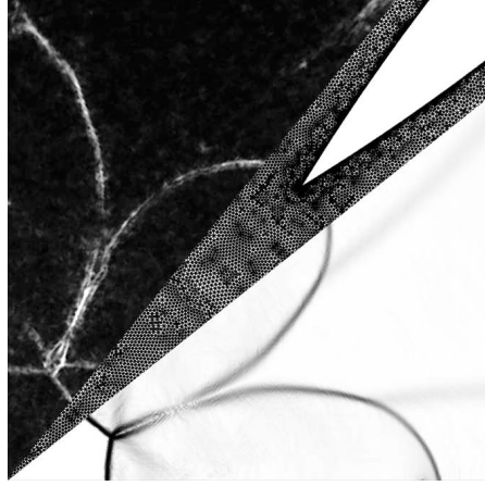
Figure 21: Comparison of a detail of a schlieren photograph Fig. 6(d), computational mesh and numerical schlieren image computed at the same instant \Delta t = -3.9 \mu s prior to implosion.
