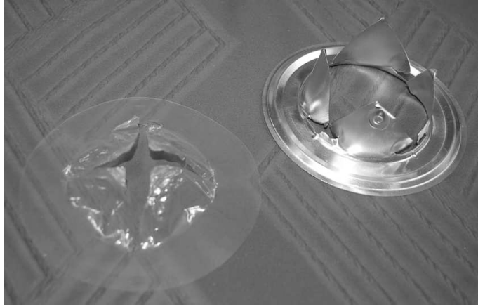
Figure 5.2: Two used membranes; one 0.05 mm plastic film and one 0.5 mm aluminium membrane. The Al membrane shows the imprint of the burst indicator on the tip of one leaf.
