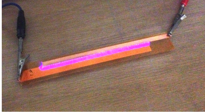
FIGURE 3.2. Photograph of the plasma produced by an in-house built single DBD plasma actuator built on the model of actuator A but with an actuation length s shorter than 140 mm.
