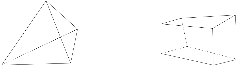
Figure 4.12: In 3D, triangular and quadrilateral elements generalize to tetrahedral (left) and hexahedral (right) meshes.
