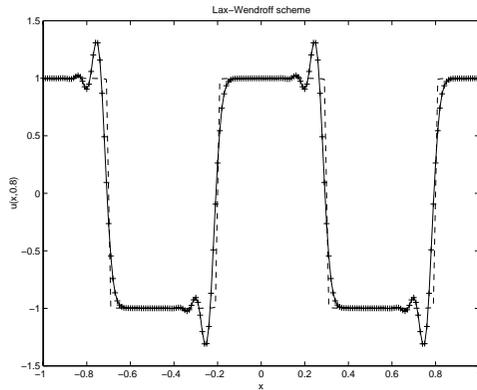
Figure 5: Numerical solution computed using Lax-Wendroff method (solid line + ) compared to the exact solution (dashed line)
