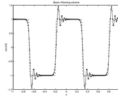
Figure 6: Numerical solution computed using Beam-Warming method (solid line + ) compared to the exact solution (dashed line)
