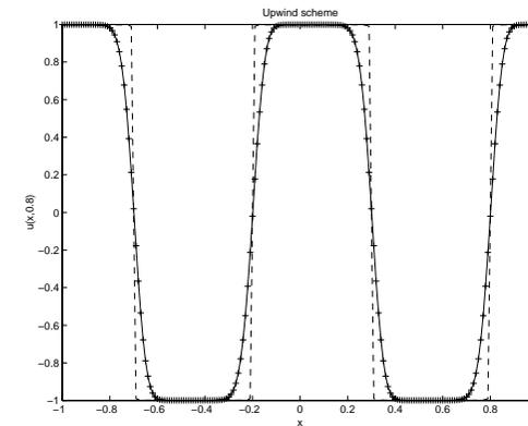
Figure 4: Numerical solution computed using Upwind method (solid line + ) compared to the exact solution (dashed line)
