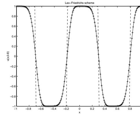
Figure 3: Numerical solution computed using Lax-Friedrichs method (solid line + ) compared to the exact solution (dashed line)
