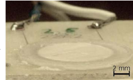
Unexpanded paste on heater
