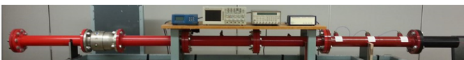
Cylindrical shock tube with a fast opening valve (FOV) and axisymmetric test chamber for spherical shock focusing
