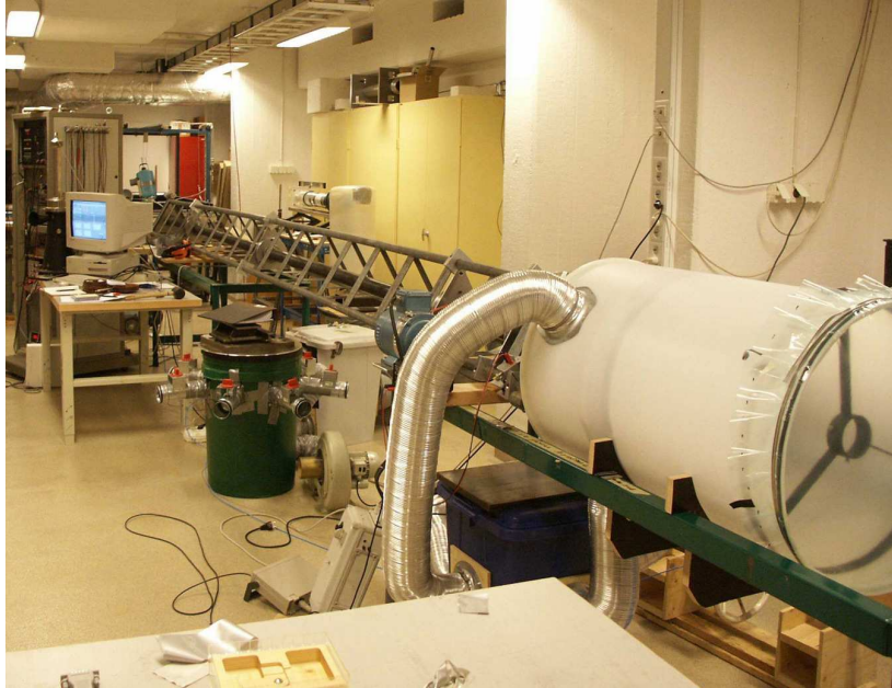
FIGURE 4.1. Experimental setup showing the pipe mounted within the triangular shaped framework and fed into the stagnation chamber covered by an elastic membrane.
