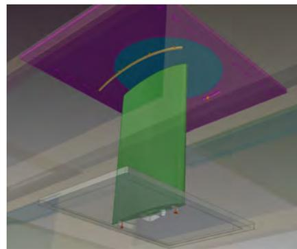
**Figure 2:** CAD drawing of the wing model mounted in the wind tunnel, with flow from right to left.
