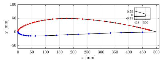
**Figure 1:** Streamwise distribution of pressure taps on a NACA 4412 airfoil profile with a chord length of 0.5 m.
