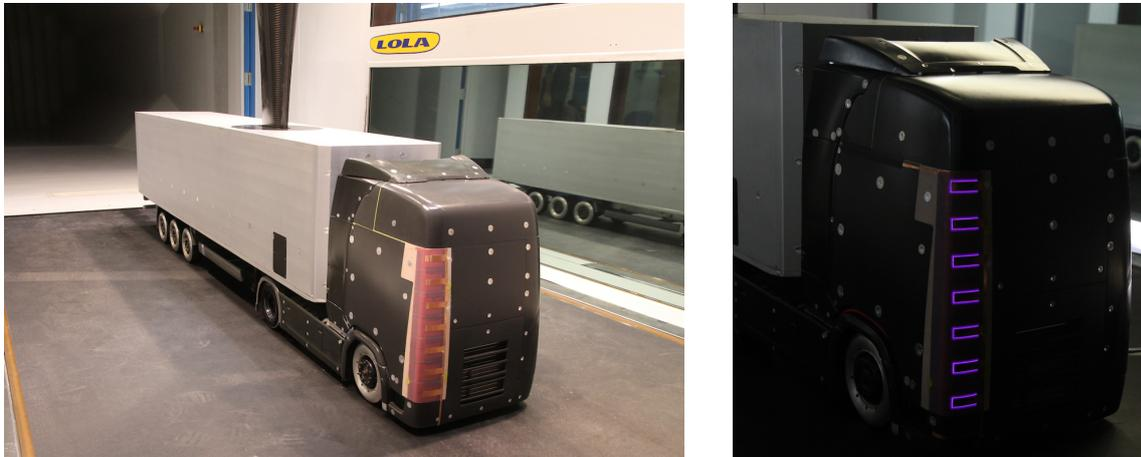
Figure 2: Picture from the wind tunnel experiments at the Lola cars aerodynamic wind tunnel [3] with the truck model equipped with an array of DBD-VGs (left image) and a zoom-in of the trailer during control (right image).
