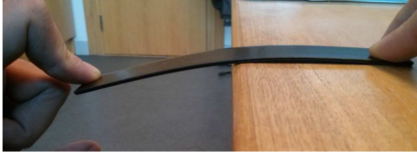
FIGURE 2.2. A deformed ruler caused by forces applied at both ends of the ruler as well as at the center of the ruler (reactive force from the table).
