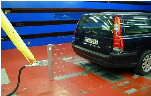
Seven-hole probe rake
