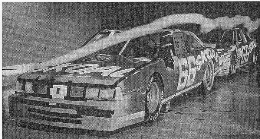
Fig. 5-34. Visualization of a smoke particle line above two Jackson NASCARs at the Lockheed wind tunnel. There is some indication that the free-stream flow does not impinge on the front grill of the following car, thus reducing its aerodynamic drag. Courtesy of Automotive Aerodynamics, Inc.
