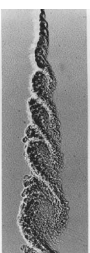
127. Coherent structure at higher Reynolds numbers. This flow is an above view at twice the pressure. Doubling the Reynolds number has produced more stable scale ratio. M. R. Kanaoka, N.A.S. Conf. Ser. of Tokyo, 1976. Photo by H. Kanaoka, 1979.
