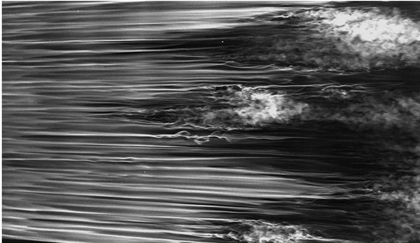
FIGURE 1. Smoke visualization of streaks and spots in a boundary layer subjected to free-stream turbulence. The white smoke is assembled in low-velocity regions and flow is from left to right. From Matsubara & Alfredsson (2001).
