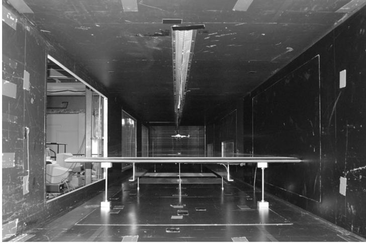
FIGURE 3.2. The test section seen from the contraction. In the ceiling the slot for the traversing system can be seen and in the center of the image the flat plate is resting on its two supporting beams.
