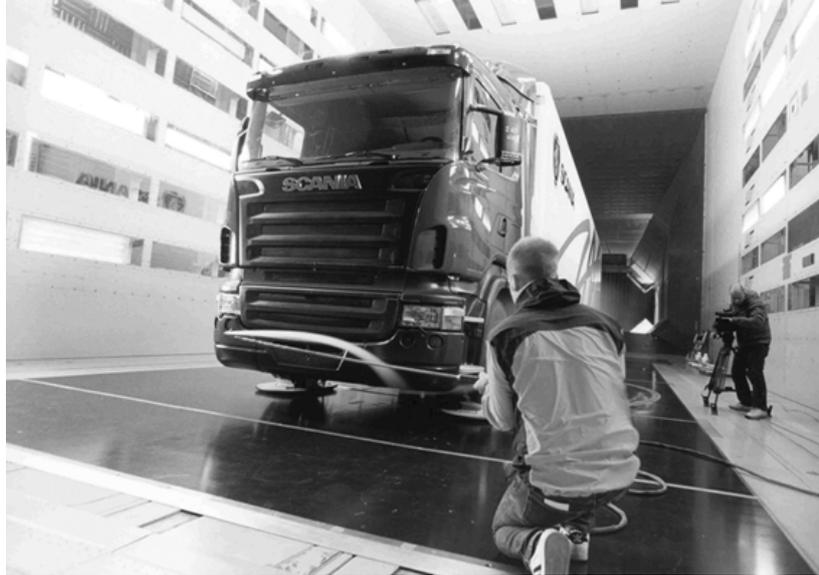
FIGURE 1.1. The author performing a smoke visualisation on a Scania truck in the German-Dutch LLF wind tunnel in 2001. The largest test section with a cross sectional area of  $9.5 \times 9.5 \text{ m}^2$  is used for this test.
