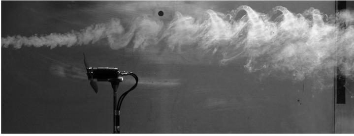
FIGURE 3.1. The smoke is introduced upstream of the rotor and captured by the tip-vortices shed from the blades, marking the helical wake boundary.
