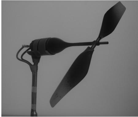
FIGURE 4.16. Model 4, rotor B as seen from upstream, *no-hub* configuration.
