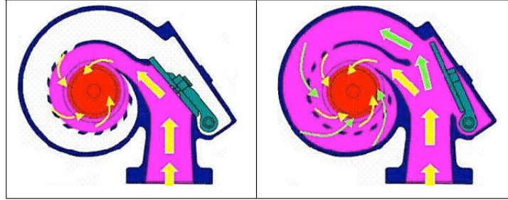
FIGURE 3.3. A Variable Geometry Turbine concept, from Andersen et al. (2006).
