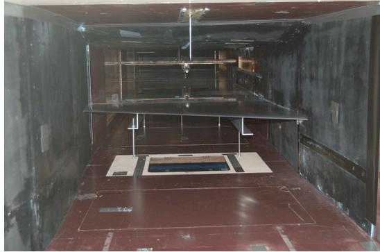
FIGURE 4.6. Photo of the completed setup in the test section. The plate is in the centre with the displacement bodies on the ceiling and walls in black. The object above the plate and reflected in the plate surface is the traversing mechanism moved far downstream.
