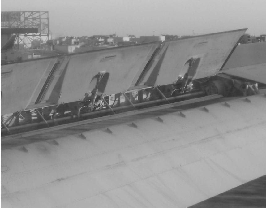
FIGURE 1.1. *Extracted flaps and spoilers uncover vortex generators on the B767-300ER flap during touch-down.*
