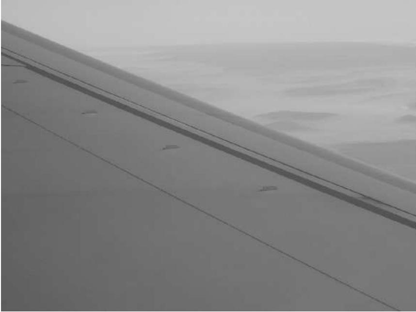
FIGURE 1.2. *Vortex generators on the main wing of a B737-800 during cruise flight.*
