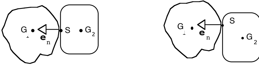
Figure 6.1: This figure illustrates some concepts presented in the text. It shows the point of impact \mathcal{S} and the normal of impact \mathbf{e}_n . The impact to the left is central and that to the right is eccentric.
