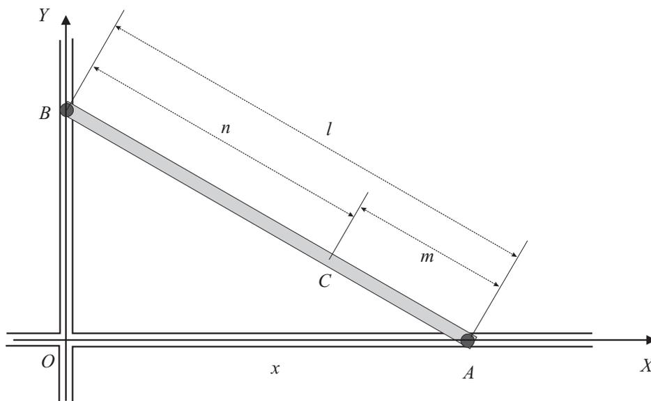
**Hints:** You could use the formula connecting the velocities of different points in a rigid body directly. It is, however, simpler to use the fact that there is pure rotation about the instantaneous center of zero velocity. You then also need the cosine theorem to get the length to  $C$ .
