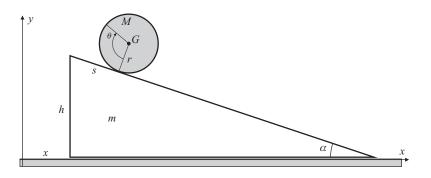
**Solution 1:** 1) Generalized coordinates: x, position of left side of the wedge, s, distance rolled by cylinder from left side of wedge. Rolling condition for cylinder:  $s = r\theta$ , where  $\theta$  is the angle that the cylinder has turned. Kinetic energy of system:
