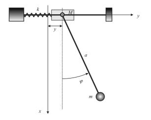
**Solution 1:** Choosing the coordinates according to the figure so that y = 0 when the spring is unloaded we find the Lagrangian
