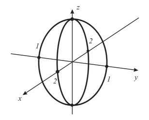
**Solution 4:** For the ring in the *yz*-plane we have  $J_x^1 = mR^2$  and since the ring is flat one must have  $J_y^1 = J_z^1 = \frac{1}{2}mR^2$ . The ring in the *xz*-plane has  $J_y^2 = mR^2$  and  $J_x^2 = J_z^2 = \frac{1}{2}mR^2$ . The total inertia tensor is diagonal and its elements are the sum of the contribution from the two rings (**Answer 1:**)
