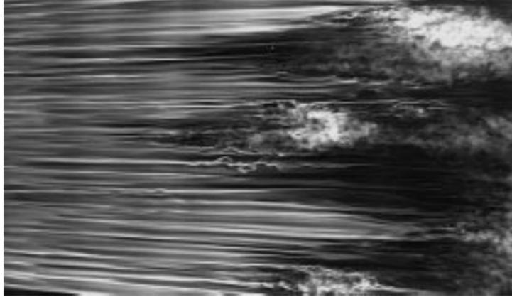
Figure 1: Flow visualization of streaky structures in boundary layers affected by free stream turbulence. Flow direction is from left to right.  $Tu=2.2\%$ ,  $U_\infty=6$  m/s.
