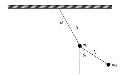
The double pendulum is the simplest dynamical system which may show chaotic behavior. In traditional education this real behavior of the double pendulum is often neglected since one immediately linearizes the equation of motions (Maclaurin expansion of the trigonometric functions and only keeping the zeroth and first order terms).
