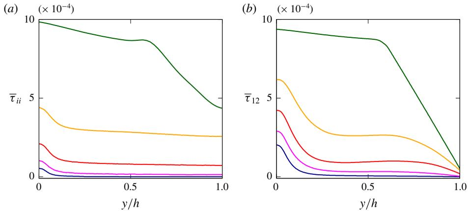
FIGURE 13. (Colour online) (a) Trace and (b) shear component of the mean elastoviscoplastic stress tensor  $\bar{\tau}_{ij}$  as a function of the wall-normal distance  $y$ . The colour scheme is the same as in figure 6.
