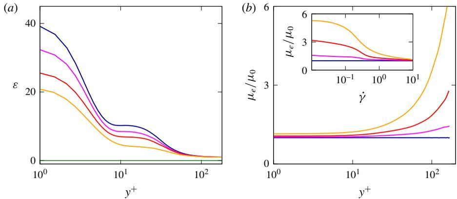
FIGURE 12. (Colour online) Wall-normal profiles of (a) the turbulent dissipation  $\varepsilon = \mu \overline{\partial u'_i / \partial x_j \partial u'_i / \partial x_j}$  in wall units and of (b) the shear effective viscosity  $\mu_e$ . The colour scheme is the same as in figure 6. The inset figure in (b) shows  $\mu_e$  as a function of the shear rate  $\dot{\gamma}$ .
