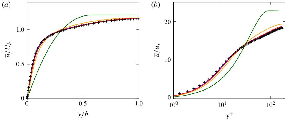
FIGURE 9. (Colour online) Mean streamwise velocity profile  $\bar{u}$  as a function of the wall-normal distance  $y$  in bulk (a) and wall units (b). The colour scheme is the same as in figure 6, with the addition of the black symbols used for the Newtonian case, taken from the results by Kim *et al.* (1987). The viscosity ratio  $\beta$  is fixed equal to 0.95.
