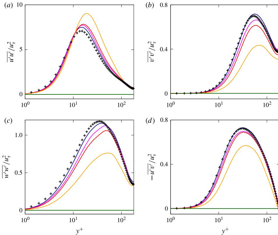
FIGURE 10. (Colour online) Wall-normal profiles of the different components of the Reynolds stress tensor, normalized with  $u_\tau^2$ . (a–c) Show the diagonal components  $u'u'$ ,  $v'v'$  and  $w'w'$ , while (d) shows the cross-term  $u'v'$ . The colour scheme is the same as in figure 6.
