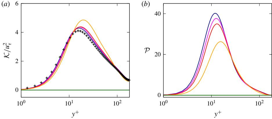
FIGURE 11. (Colour online) Wall-normal profiles of (a) the turbulent kinetic energy  $\mathcal{K} = (u'^2 + v'^2 + w'^2)/2$  and of (b) the turbulent production  $\mathcal{P} = -\overline{u'v'} d\bar{u}/dy$ , both normalized with the friction velocity  $u_\tau$ . The colour scheme is the same as in figure 6, with the blue, magenta, red, orange and green colours used for the turbulent cases with  $Bi = 0, 0.28, 0.7, 1.4$  and  $2.8$ , respectively.
