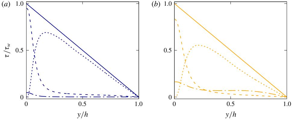
FIGURE 14. (Colour online) Normalized shear stress balance across the channel, for (a)  $Bi=0$  and (b)  $Bi=1.4$ . The dashed, dotted and dash-dotted lines are used for the viscous, Reynolds and elastoviscoplastic shear stress, respectively, while the solid line is the total shear stress, which varies linearly across the channel height.
