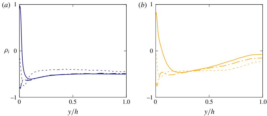
FIGURE 15. (Colour online) Wall-normal profiles of the cross-correlations  $\rho_i$  of the streamwise (dashed line), wall-normal (solid line) and spanwise (dash-dotted line) velocity component  $u_i$  and elastoviscoplastic contribution  $f_i$ , defined in (3.5), for (a)  $Bi=0$  and (b)  $Bi=1.4$ .
