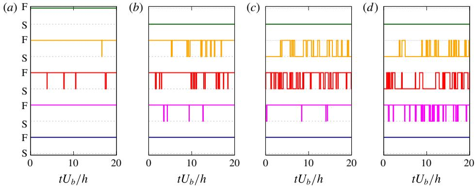
FIGURE 8. (Colour online) Intermittency of the yield/unyield process (F/S) as a function of time. The four panels correspond to probes located at  $x = 3h$ ,  $z = 1.5h$  and different wall-normal distances: (a)  $y \approx 0.25h$ , (b)  $0.49h$ , (c)  $0.74$  and (d)  $0.98h$ . The lines in every panel are the results with different Bingham number, with the colour scheme being the same as in figure 6.
