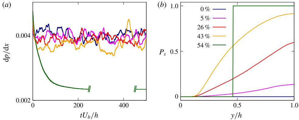
FIGURE 6. (Colour online) (a) Time history of the streamwise pressure drop  $dp/dx$  for different Bingham numbers  $Bi$ . (b) Probability of the fluid being unyielded  $P_s$  as a function of the wall-normal distance  $y$ . The percentages reported in the legend show the mean unyielded volume  $Vol_s$ . The blue, magenta, red, orange and green colours are used for  $Bi = 0, 0.28, 0.7, 1.4$  and  $2.8$ , respectively. The viscosity ratio  $\beta$  is fixed equal to  $0.95$ .
