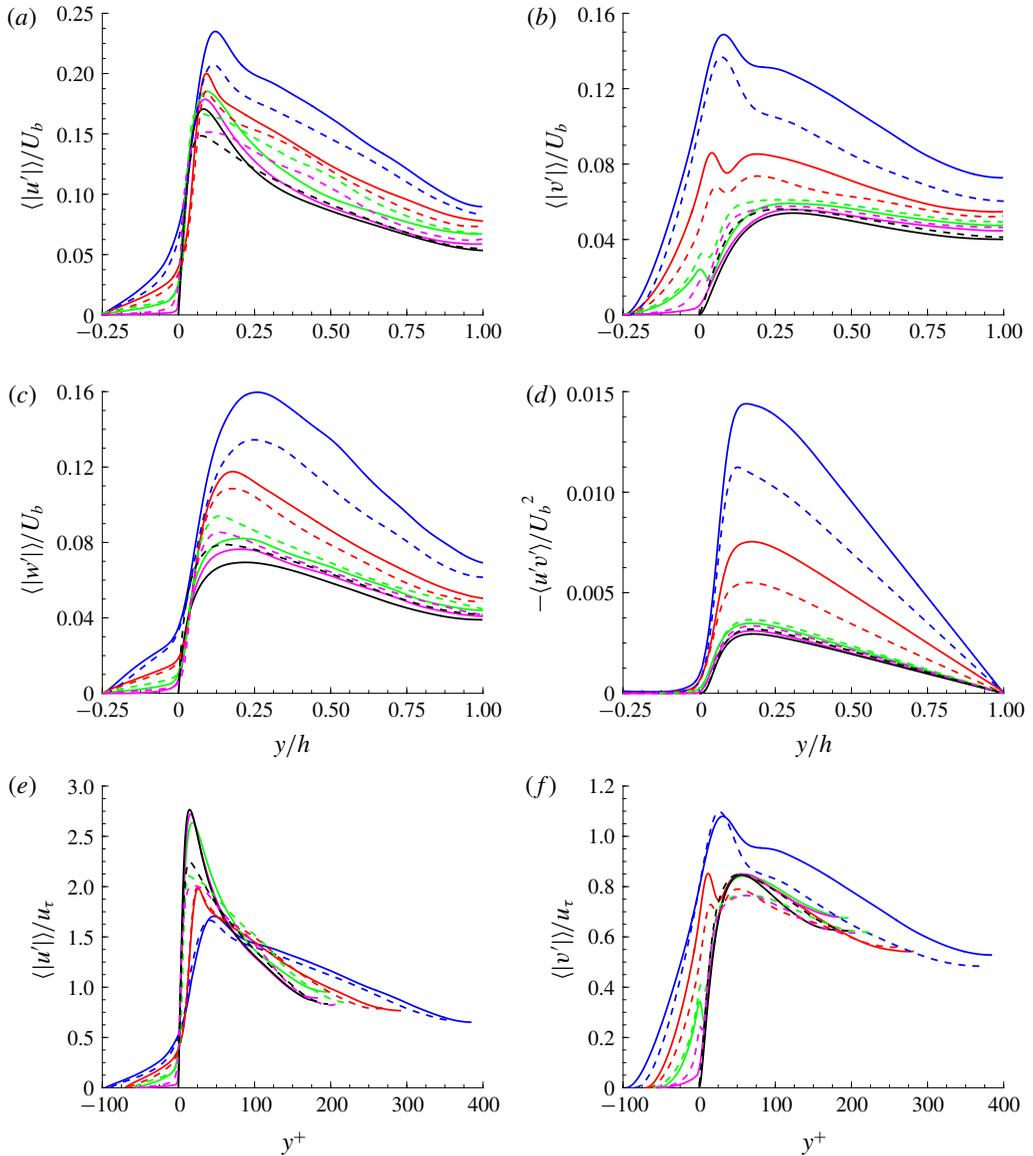
FIGURE 5. (Colour online) Root-mean-square velocity fluctuations and Reynolds shear stress: (a) streamwise  $\langle |u'| \rangle$ ; (b) wall normal  $\langle |v'| \rangle$ ; (c) spanwise  $\langle |w'| \rangle$  and (d) Reynolds shear stress. Panels (e) and (f) show  $\langle |u'| \rangle$  and  $\langle |v'| \rangle$ , scaled in internal units. The colour scheme is the same as in figures 2 and 3(a).
