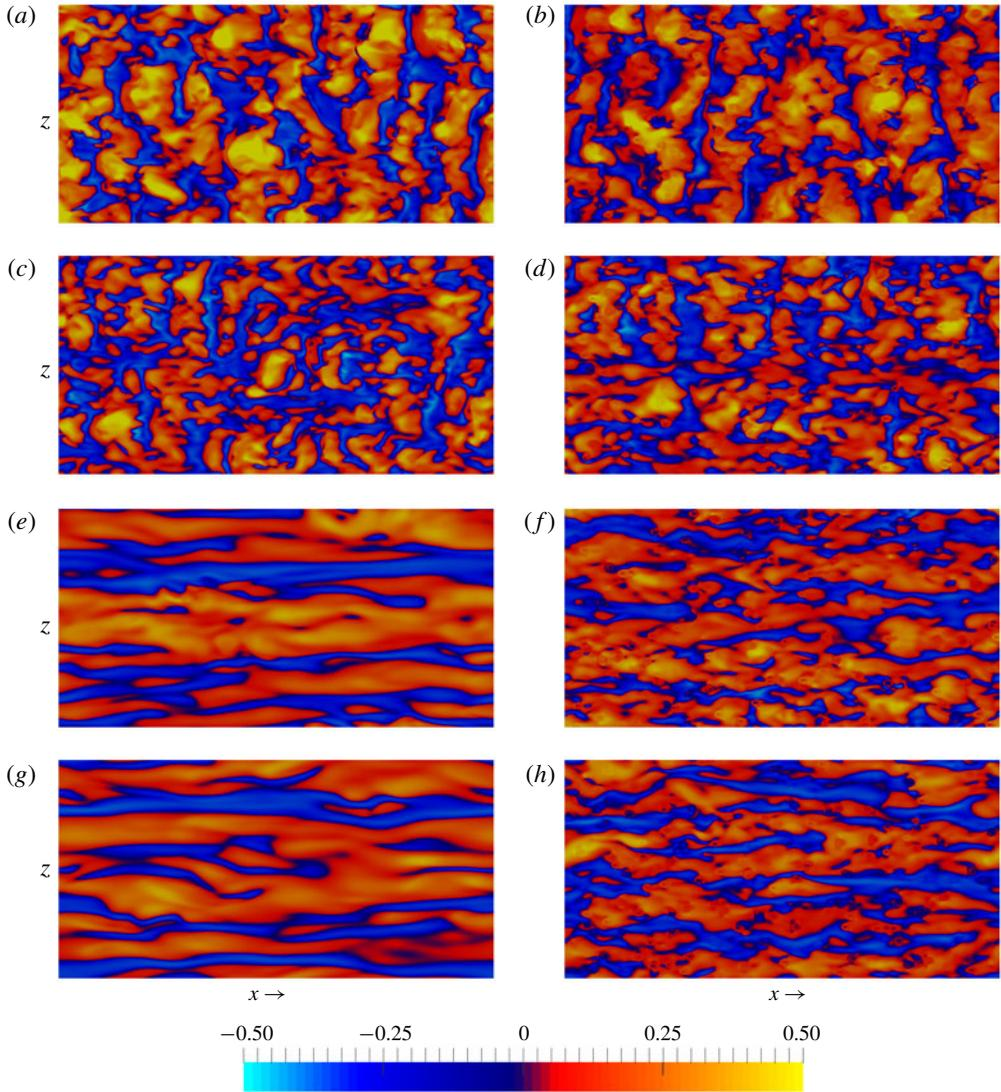
FIGURE 6. (Colour online) Instantaneous contours of the streamwise velocity fluctuations  $u'$  in the wall-parallel plane  $x-z$  at  $y/h=0.1$ . The colour scale goes from  $-0.5U_b$  (blue) to  $0.5U_b$  (yellow). (a,c,e,g) indicates the single-phase flow cases ( $G1$  to  $G4$ ) and (b,d,f,h), the particulate ones ( $G1_{10\%}$  to  $G4_{10\%}$ ), with  $G^*$  increasing from (a–h).
