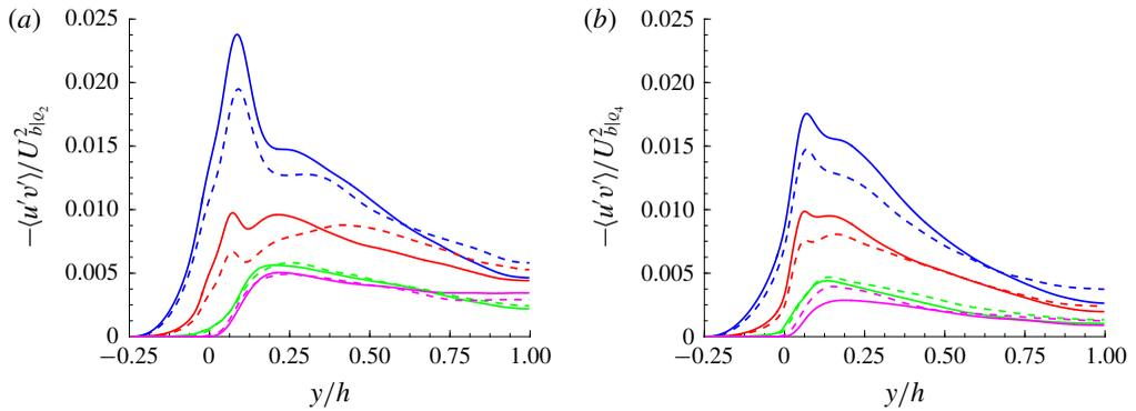
FIGURE 9. (Colour online) Reynolds shear stress, conditionally averaged for (a) the second ( $Q_2$ ) and (b) the fourth ( $Q_4$ ) quadrant of  $u'-v'$  plane.
