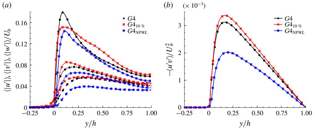
FIGURE 11. (Colour online) (a) Root-mean-square velocity fluctuations  $u'$ ,  $v'$  and  $w'$  in the streamwise, —, wall-normal, - - - and spanwise, . . . , directions and (b) Reynolds shear stress, scaled in outer units for the cases  $G4$ ,  $G4_{10\%}$  and  $G4_{NPWL}$ .
