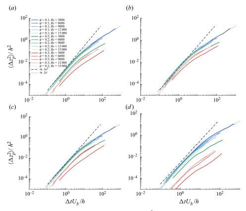
Figure 9. Single-particle mean-square spanwise displacement,  $\langle \Delta z_p^2 \rangle (\Delta t, y)$ , normalized with the half-channel height,  $h^2$ , averaged over (a) the whole domain and for particles initially ( $\Delta t = 0$ ) located at (b)  $0 < y_p < h/3$ , (c)  $h/3 < y_p < 2h/3$  and (d)  $2h/3 < y_p < h$ .
