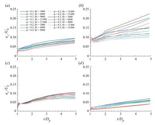
Figure 12. Collision kernel,  $\kappa_c(r) = g(r) \cdot \Delta V_p^{n,-}(r)$ , averaged over (a) the whole domain and over particles located in (b)  $0 < y_p < h/3$ , (c)  $h/3 < y_p < 2h/3$  and (d)  $2h/3 < y_p < h$ .
