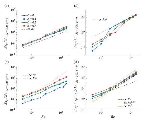
Figure 8. (a) The viscous stress,  $\Sigma \tau_V$ , (b) the turbulent stress,  $\Sigma \tau_T$ , (c) the particle-induced stress,  $\Sigma \tau_P$ , and (d) the total stress,  $\Sigma (\tau_V + \tau_T + \tau_P)$ , normalized by the total stress in the laminar single-phase flow, as a function of the Reynolds number; the data pertaining to  $Re \in [500-2000]$  are adapted from Yousefi et al. (2021).
