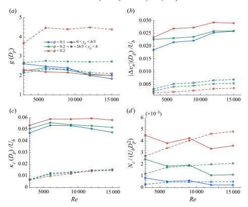
Figure 13. (a) The RDF, (b) magnitude of the relative approaching velocity and (c) collision kernel at contact  $(r = D_p)$ , together with (d) collision frequency,  $N_c = \pi \langle \Phi \rangle^2 D_p^2 \kappa_c(D_p)$ , vs the Reynolds number for different volume fractions. Solid lines denote averaging over particles located at  $0 < y_p < h/3$  and dashed lines  $2h/3 < y_p < h$ .
