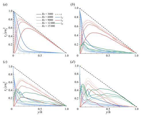
Figure 5. Momentum budget for the different bulk volume fractions: (a) single phase, (b)  $\phi = 0.1$ , (c)  $\phi = 0.2$  and (d)  $\phi = 0.3$ . Here,  $\tau$  is the total stress,  $\tau_V$  denotes viscous stress,  $\tau_T$  the turbulent Reynolds shear stress of the combined phase and  $\tau_P$  the particle-induced stress.
