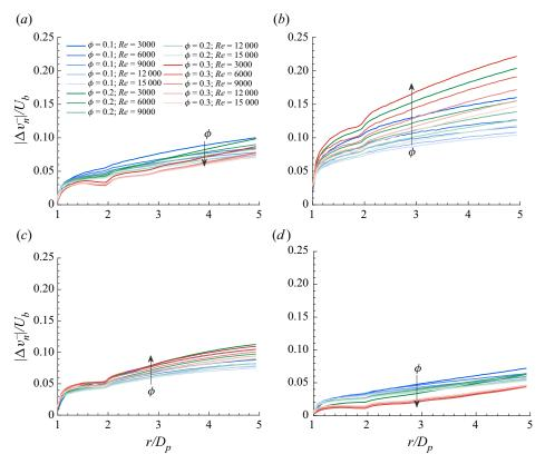
Figure 11. Magnitude of relative approaching normal velocity,  $|\Delta v_n^-|$ , averaged over (a) the whole domain and particles located in (b)  $0 < y_p < h/3$ , (c)  $h/3 < y_p < 2h/3$  and (d)  $2h/3 < y_p < h$ .
