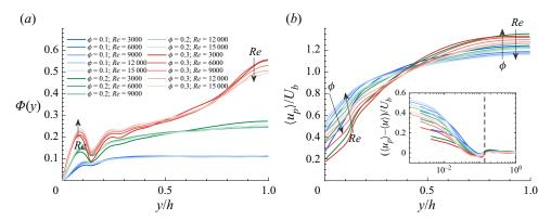
Figure 4. (a) Profiles of the local solid volume fraction as a function of the wall-normal distance. (b) Outer-scaled mean streamwise particle velocity profiles; the inset shows the apparent particle-to-fluid slip velocity,  $\langle u_p \rangle - \langle u \rangle$ , in semi-logarithmic scale, while the vertical dashed line indicates the wall-normal distance corresponding to one particle diameter.
