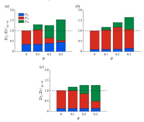
Figure 7. The contribution of the viscous,  $\Sigma \tau_V$ , Reynolds,  $\Sigma \tau_T$ , and particle-induced stress,  $\Sigma \tau_P$ , for different solid volume fractions at (a) Re = 3000, (b)  $Re = 15\,000$  and (c) Re = 9000. Each contribution is integrated across the channel and normalized by the total stress of the single-phase flow with the same bulk Reynolds number.
